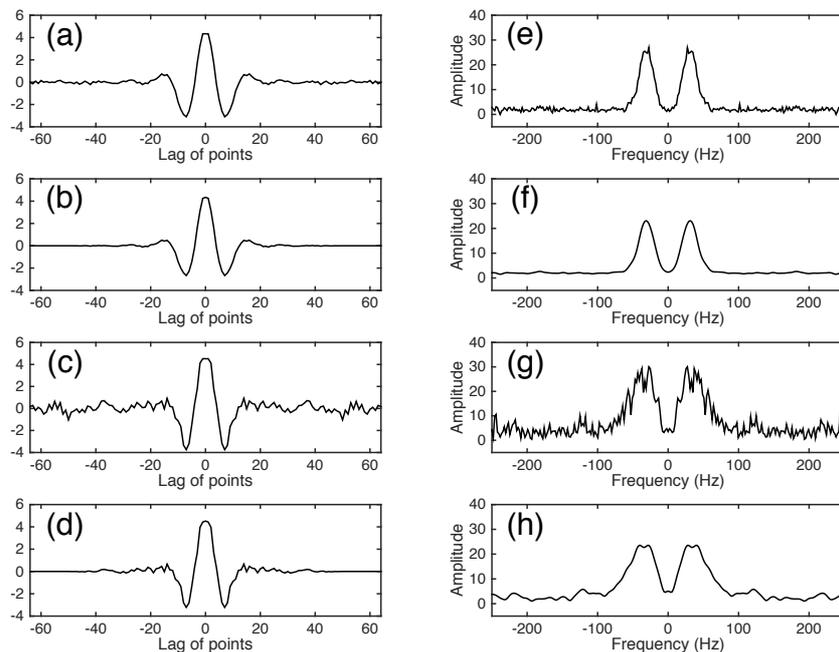
**Figure 2** Designed filter for (a)  $\sigma = 0.3$ , without truncation; (b)  $\sigma = 0.3$ , with truncation; (c)  $\sigma = 0.6$ , without truncation; (d)  $\sigma = 0.6$ , with truncation. The truncation windows length is 100 sample points. And frequency response of the filters (e)  $\sigma = 0.3$ , without truncation; (f)  $\sigma = 0.3$ , with truncation; (g)  $\sigma = 0.6$ , without truncation; (h)  $\sigma = 0.6$ , with truncation.
