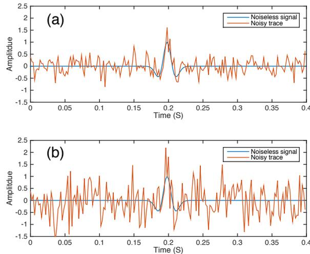
**Figure 1** Noiseless and noisy traces, (a)  $\sigma = 0.3$ ,  $SNR = -6.03$  dB; (b)  $\sigma = 0.6$ ,  $SNR = -12.01$  dB.
