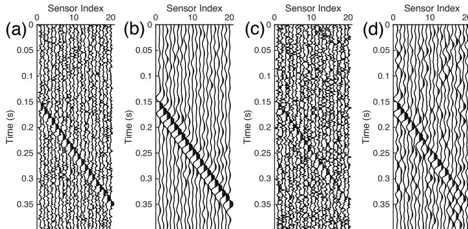
**Figure 3** (a) noisy traces, only show 20 traces,  $\sigma = 0.3$ ; (b) denoising result of the  $\sigma = 0.3$  case; (c) noisy traces, only show 20 traces,  $\sigma = 0.6$ ; (d) denoising result of the  $\sigma = 0.6$  case.
